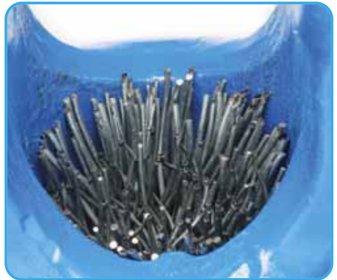
Figure 5: Properly positioned broom with the wire ends protruding slightly.
