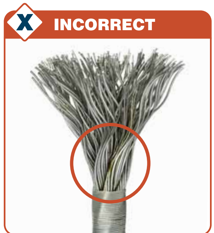
Figure 4: Incorrectly broomed wire rope.
