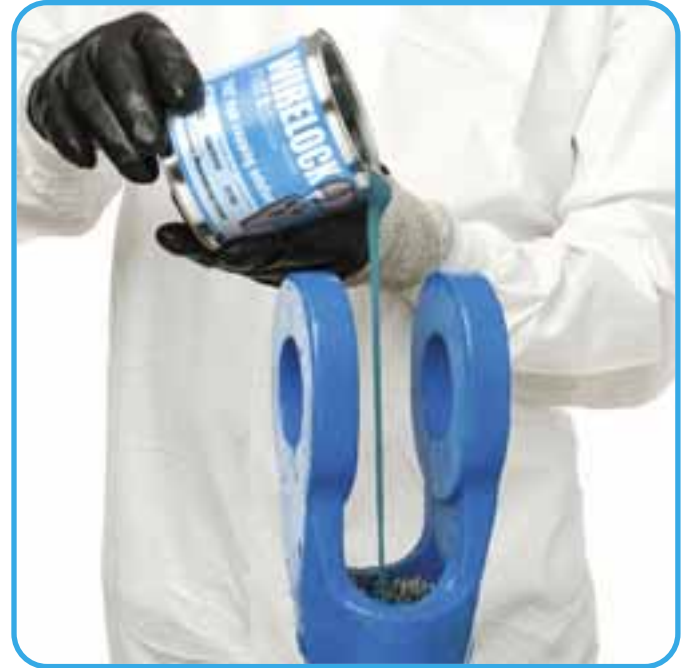
Figure 9: Upon mixing the compound should be poured immediately.
