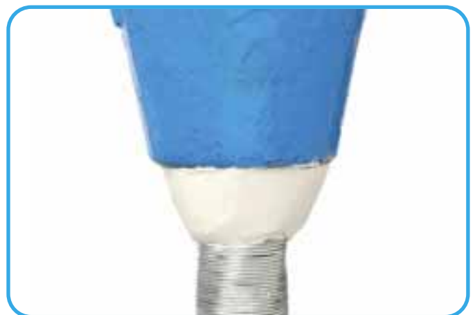
Figure 7: Axes of socket and rope properly aligned and sealed with WIRELOCK putty/ clay.
